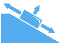
Inclined Plane - Like a lever, this is usually used to move heavy objects. It has a gently sloped surface so that objects can be moved up with less force. How might this be used to get Rapunzel down? Think about the force that would be exerted going down.
